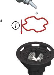
NOTE: The diff assembled as shown here, should weigh max 17.1 grams
